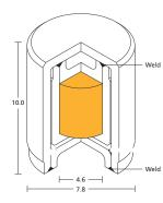
Sources up to  $500 \mu g$  can be manufactured in the X1 capsule design. Outer capsules are available in stainless steel or zircalloy:
