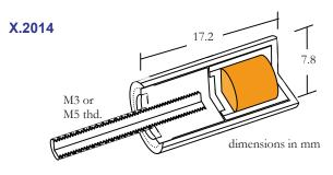
The X.2014 is an extended X.1 capsule with a female M3 threaded lid. An M3 (X.2014) or M5 (X2014/1) handling rod can be provided. Activities are available up to 8GBq (400 µg).
