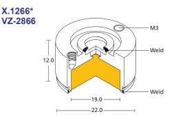
\* X.1266 manufactured according to drawing VZ-2866
